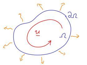
This is the heat exchanger configuration: given an initial distribution of heat, it is fluxed away through the cooled boundaries.
