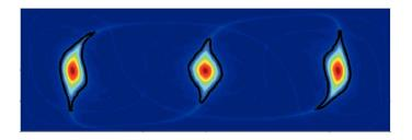
The islands are made to follow the  $\sigma_2 \sigma_1^{-1}$  stirring protocol by clever wall motions! (viscous Stokes flow)
