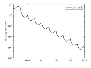
Notice that variance (solid line) shows significant oscillations. Fitting a decay rate to this, or trying to optimize, is more challenging than it needs to be.
