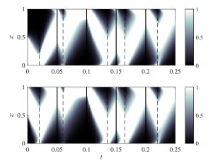
Two different initial conditions converge to the same aperiodic solution  $\varphi(\boldsymbol{x},t)$ .
