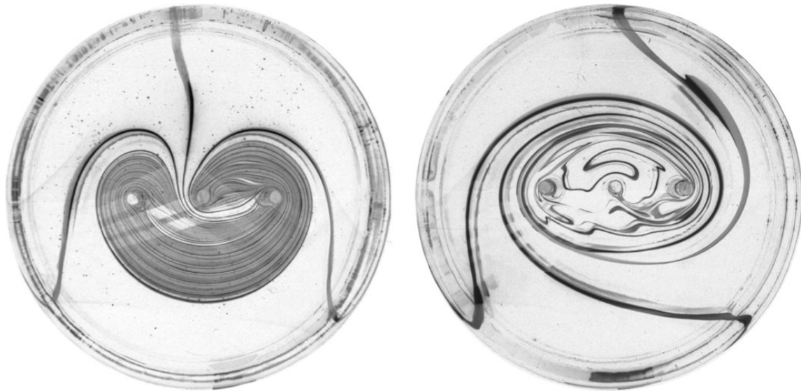
Fig. 2.8 Experimental stirring device with three rods immersed in a viscous fluid. Left: motion corresponding to \bar{T}_2^{-1}\bar{T}_1 . Right: motion corresponding to \bar{T}_2\bar{T}_1 . The black dye suggests how the fluid is displaced. (From Boyland et al [9].)
