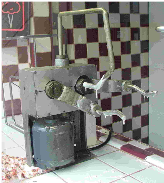
Fig. 2.1a A taffy-pulling device (from Finn and Thiffeault [12]).
