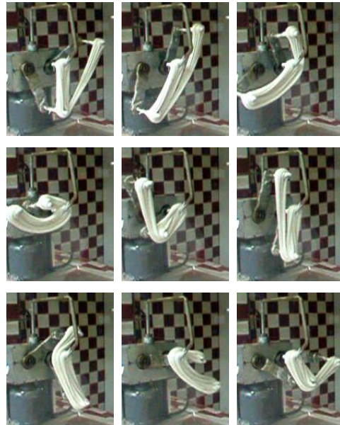
Fig. 2.1b Snapshots over a full period of operation, with taffy (from Finn and Thiffeault [12]).
