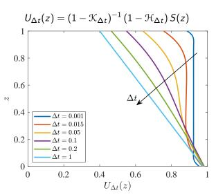
Rapid flipping gives constant interior temperature with boundary layers.
