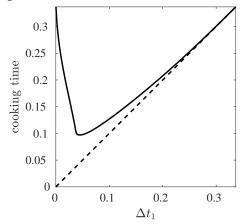
Notice the asymmetry of the minimum: it is better to err on the right. Minimum  $t_{cook}$  is 0.0970 (80.5 s) with a flip at 0.0436 (36 s).
