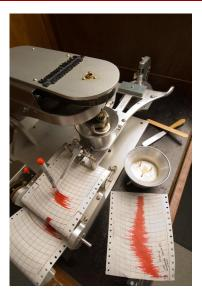
The mixograph measures the resistance of the dough to the pin motion.
