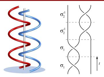
The three rods of the taffy puller in a space-time diagram. Defines a braid on n=3 strings,  $\sigma_1^2 \sigma_2^{-2}$  (three periods shown on the left).
