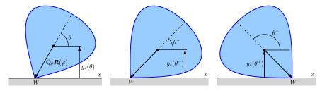
The angle  $\theta$  can vary from the right-tangency angle  $\theta^-$  to the left-tangency angle  $\theta^+$ .
