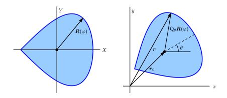
Convex swimmer in its frame (X, Y) and the fixed lab frame (x, y).
