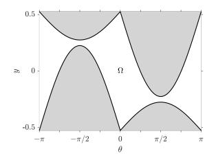
Configuration space for the needle in of length  $\ell = 1$  in an open channel of width L = 1.05. (x not shown.)
