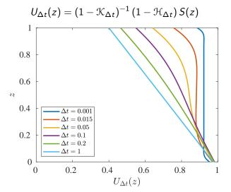
Rapid flipping gives constant interior temperature with boundary layers.
