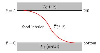
Plot temperature profiles with z on the vertical and T on the horizontal.
