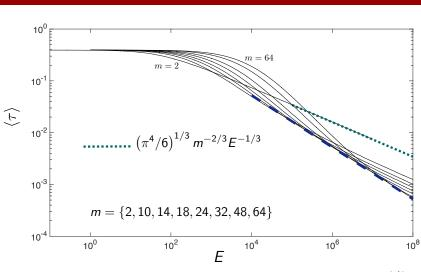
Fixed-*E* asymptotic optimal  $\langle \tau \rangle$  seems to decrease to zero as  $m^{-2/3}$ . This implies no optimal flow, since arbitrarily efficient at large *m*. Not so!
