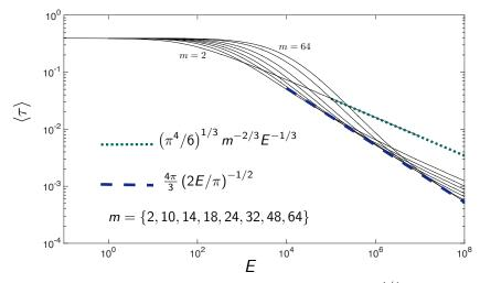
To truly capture the optimal solution, have to let  $m \sim E^{1/4}$ . This is the dashed line (envelope).
