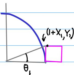
$$\begin{aligned} T_3 &= \int_{\theta_1}^{\pi/2} \left( \frac{1}{u} + 1 \right) \frac{dx}{d\theta} d\theta \\ &= \frac{1}{2} \int_{\theta_1}^{\pi/2} \frac{\cos 2\theta}{\sin \theta} d\theta , \quad \theta_1 \text{ small.} \end{aligned}$$
