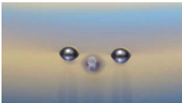
Fig. 1 Three paramagnetic beads afloat on a meniscus. Reproduced from Lumay et al. , 48 with permission from The Royal Society of Chemistry.
