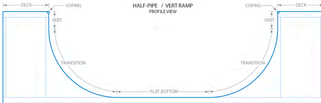
Figure 1. End-on schematic view of a half-pipe. (Source: Wikimedia Commons; created by Dennis Dowling.)
