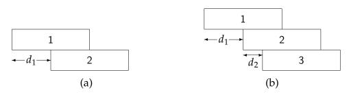
In diagram (a), the bricks will be stable as long as the center of mass of brick 1 does not overhang the edge of brick 2, and thus  $d_1 = 1/2$ .
