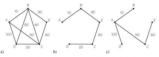
Each is an example of a minimal **subgraph** connecting all the vertices in the original. In each case, removal of any edge will disconnect the graph.
