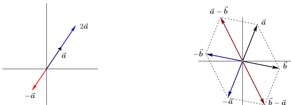
Figure 16: Multiples of a vector, and the difference of two vectors.
