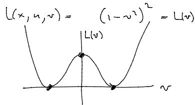
$$\begin{aligned} \text{Euler-Lagrange Eqn: } \frac{d}{dx} \left( \frac{\partial L}{\partial v} \right) &= \frac{\partial L}{\partial u} \Leftrightarrow \frac{d}{dx} \left( 2u'(x)(1-u'(x)^2) \right) = 0 \\ &\Leftrightarrow u''(x)(1-u'(x)^2) - 2u'(x)^2 u''(x) = 0 \\ &\Leftrightarrow u''(x)(1-3u'(x)^2) = 0 \\ &\Leftrightarrow u''(x) = 0 \quad \text{or} \quad u'(x) = \pm \frac{1}{\sqrt{3}} (\approx \pm 0.57...) \end{aligned}$$
